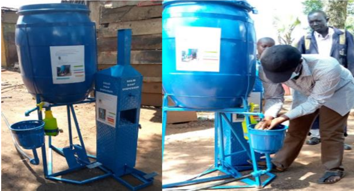
Image 2 A mechanised free touch hand washing equipment innovated by a technician at Kyambogo University June, 2020
